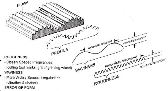
Long Period or Non-cyclic Deviations (errors in ways or spindles, uneven wear)
