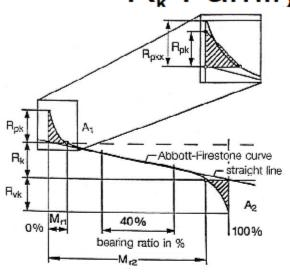
Material filled profile peak area Lubricant filled profile valley area Core roughness depth Reduced peak height Reduced valley depth Material component relative to peaks Material component relative to valleys R<sub>pkx</sub> (R<sub>pk</sub>\*) R<sub>vkx</sub> (R<sub>vk</sub>\*) Total Peak Height Total Valley Depth
