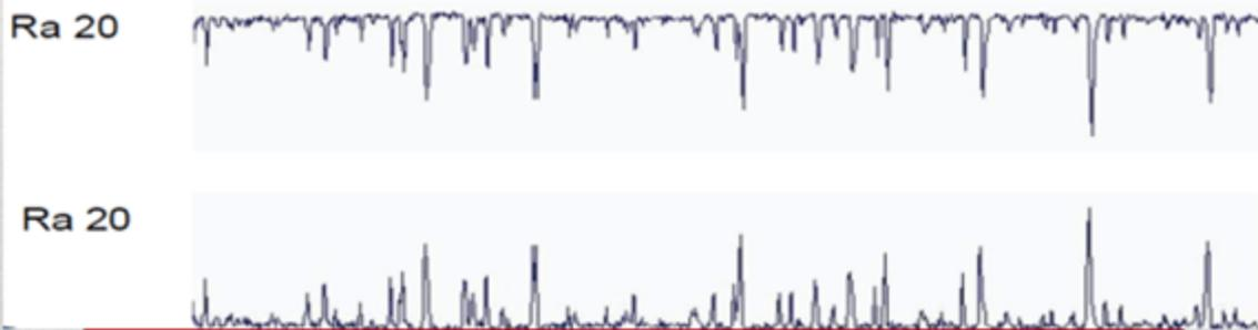
For a clear and accurate understanding of plateau cylinder wall finishes we use the Rk family of parameters. These included RpK, Rvk and Rk which help define the proper surface finish or plateau finish we need for the application the engine is being used in. The example here shows the main three parameters used in plateau finish measurements.
