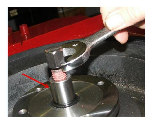
Do not overheat. Be cautious using a flame near the table lubricant. And allow to cool fully before inserting a new E-Z Lok.
