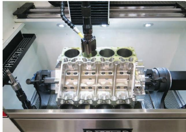
Odd shaped blocks such as the Subaru "Boxter" are set up easily. All cylinders are Automatically honed in one cycle with the efficiency of unattended operation.
